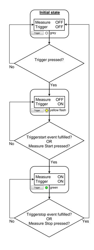
In the previous signal flowchart, the general course of measurement by means of a triggering is described. The activation button 'Trigger' can be found in the 'Meas./Diagram Mode' under 'Measure Stop'. The software triggering consists of two events which are adjustable according the requirements as follows:
